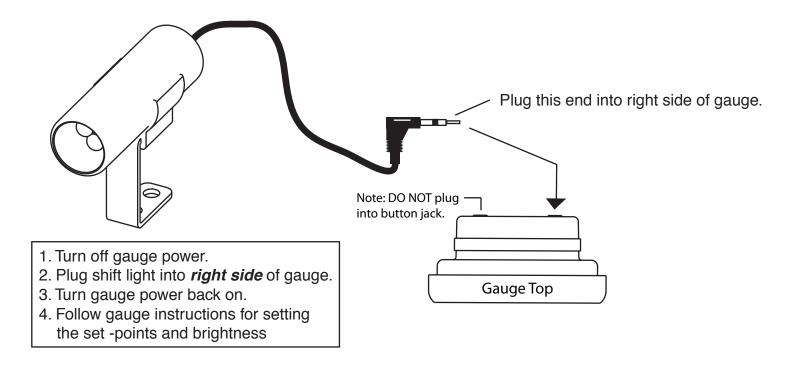
**OPTIONAL SETUP**: If you wish to use the Shift-Light/Warning-Light in a different application then you do have the option to connect it directly to a 12volt source to power on the LEDs.
