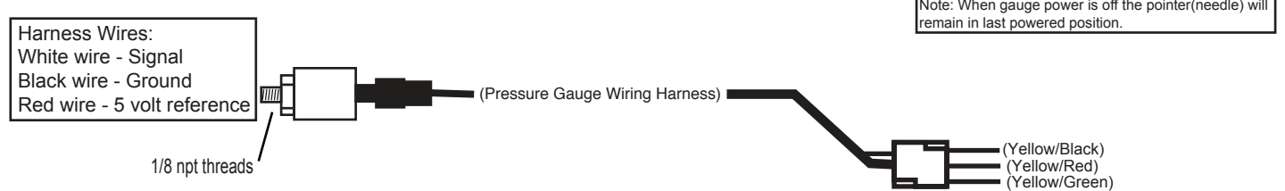
FIGURE 8: Pressure Sensor Connection
