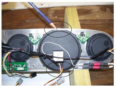
15. The top and bottom of the tachometer spin ring will require modification to help clear the binnacle housing.
