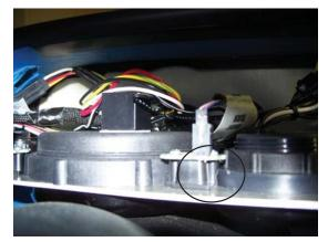
13. The right turn signal could interfere with adjacent spacer ring. Use a dremel tool to remove material off the spacer ring. Very minimal material removal is all that is necessary.
