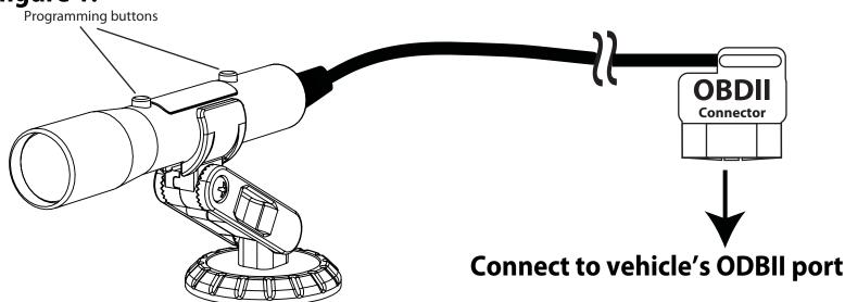
OBDII NOTE: Speedhut SST-MAX Shift-light will not function when used in conjunction with any other OBDII device.
