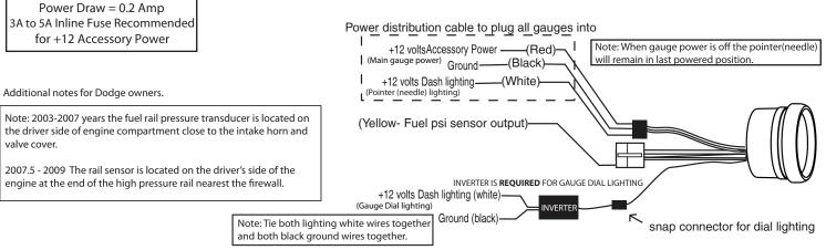
\*\*\*Protect any unused connectors. Damage to an unused connector could cause inverter failure.\*\*\*
