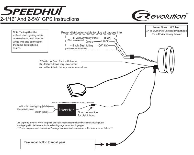
1. Hook up speedometer power requirements as shown above.
